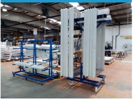
Build trolleys to materials that are difficult to transport, assuring no damages or scratches
