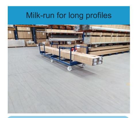
Long aluminium profiles (6m / 20ft) were now simple to deliver to cutting machine
