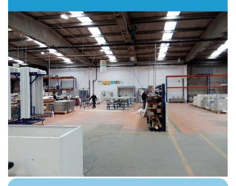
Remove pallet racking storage => material needs to flow + less use of forklifts
